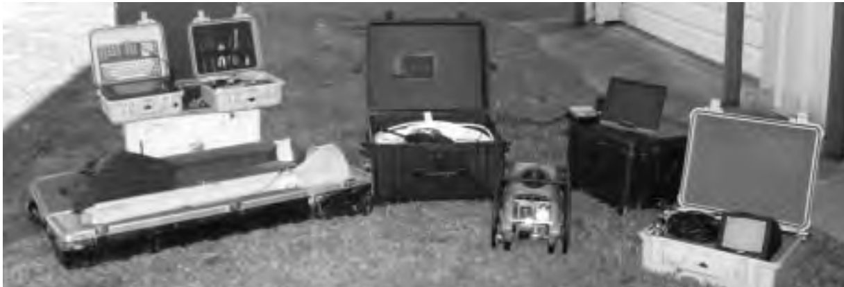
This equipment, used in the anthrax underwater search investigation, allows investigators to image the bottom of the body of water and help locate items that could potentially be crime-related.
